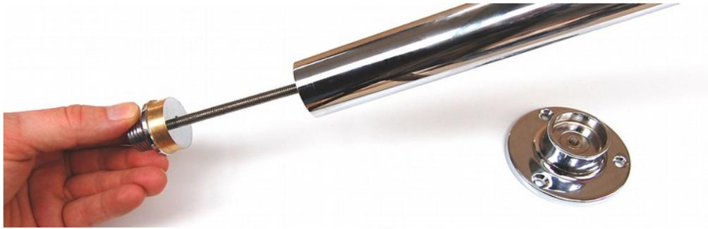
5. Now remove the internal threaded stud by unscrewing it.
