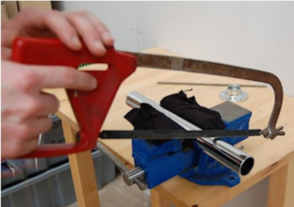
7. Now the stud needs to be cut down by the same amount as the tube. Measure the piece of tube you have just removed and mark this length on the threaded stud, cut this off using a hacksaw. De-burr the end of the stud so the nut screws over with ease. See **Fig.7**
